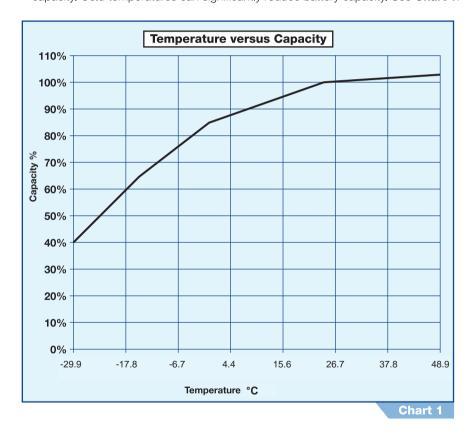
Although higher temperatures increase the battery capacity they also accelerate corrosion and reduce overall battery life. For example, batteries operating continuously at 100°F (37.8°C) could experience as much as 25% reduction in life.
