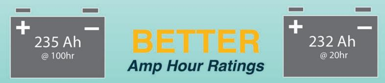
Amp hour ratings are often used to compare batteries, but not all Ah ratings are taken at the same discharge rate (10-hr, 20-hr, etc.). Batteries that show the same ratings may be completely different, as the advertised discharge rates may be higher for one rating and lower for another.
